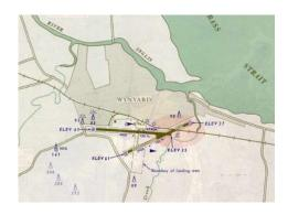
The diagram above from the 15 March 1968 Landing Chart shows the airport layout with the rail crossing highlighted. Interestingly, the chart contains a note (not shown) that the runway lights on the northern side of Runway 08/26 can be confused with parallell street lights (Runway 05/23 was not lit for night flying).
