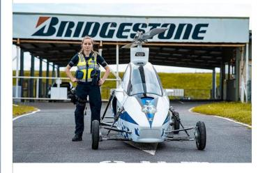
The Pegasus E 'flying car' is an Aussie invention that can be driven like a car and flown like a helicopter, giving it greater scope – namely, to take to the air – during high-speed vehicle pursuits, which police forces are increasingly prohibiting due to safety concerns.
